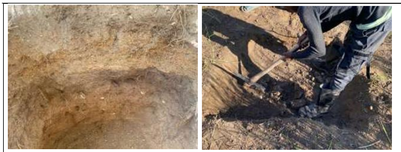
Figure 12 Images of toe samples taken from road edge by design consultant LASA, April 2024
